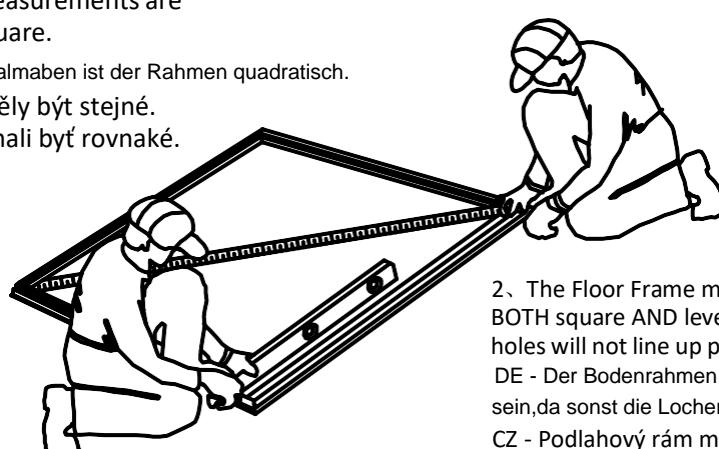
2、The Floor Frame must be BOTH square AND level or the holes will not line up properly.
